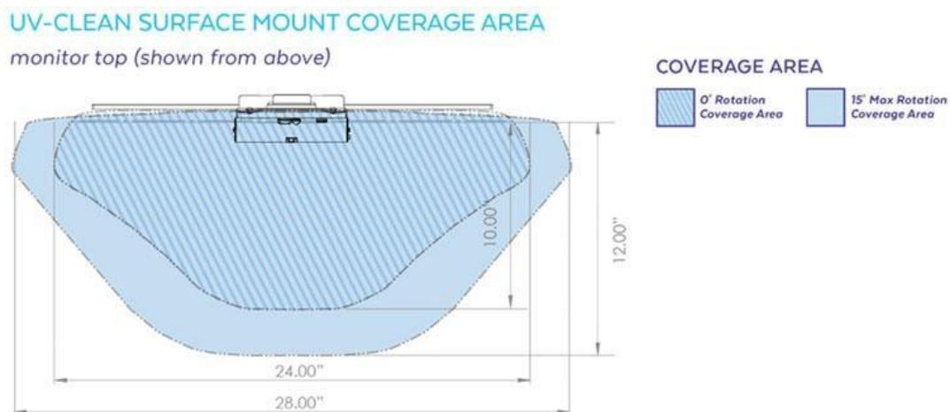
Figure 1. UV-CLEAN Surface Mount configuration attaches to the top of any monitor bezel.
